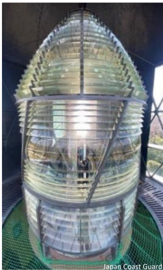
Second-Order Fresnel lens, installed in 1884
